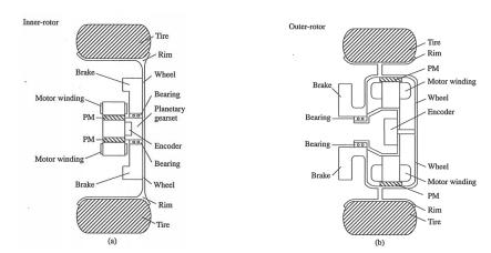
Compare the operational differences and their advantages/disadvantages of the above two in-wheel motor.
